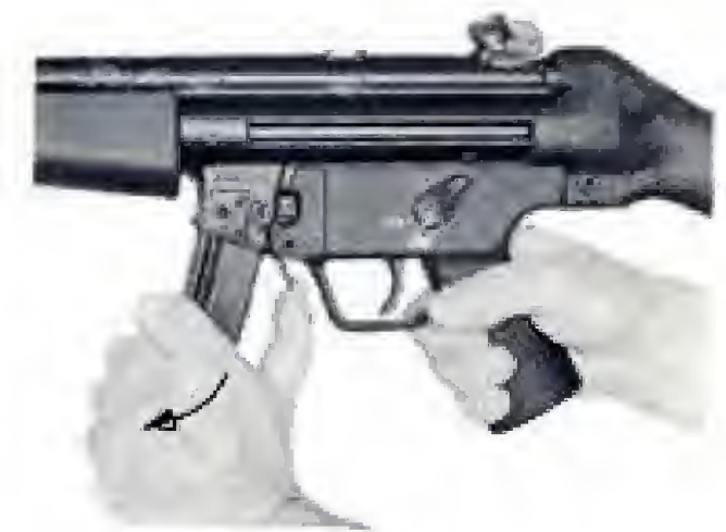
Fig. 28 Removing the magazine
